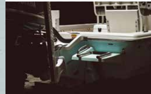
Swim ladder and platform
